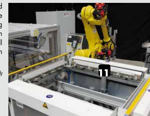
GEROLD station for frame assembly
