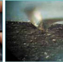
Cross section of a laser engraving with 0,2 mm engraving depth
