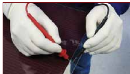
Decisive criterion for edge deletion is insulation testing
