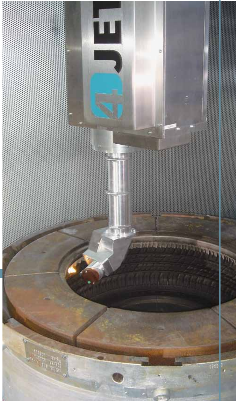
Cleaning of a tire mold with laser
